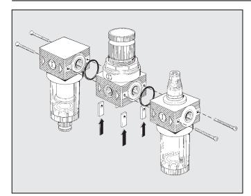
Use ASSEMBLY PLATES (code 9170201) to assemble the Bit elements correctly.
