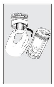
To clean or replace the filter element unscrew the screen of the centrifuge assembly. Use a no. 3 compass spanner to unscrew the bowl.
