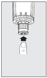
Press the button to drain condensate when the bowl is pressurized.
