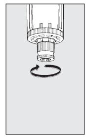
Turn the knob anticlockwise to close the valve with bowl pressurized or not pressurized.
