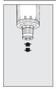
With the knob in the centre position, the drain is semiautomatic. The drain operates when the bowl is not pressurized and closes when it is.
